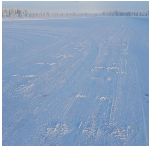
Figure 6. Snow-plough effect observed during braking.
